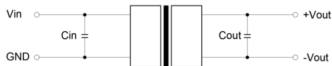
Figure 1: Typical External circuit
